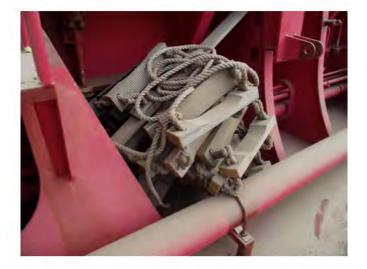
Typical storage of Pilot ladder on a handy size bulk carrier.
